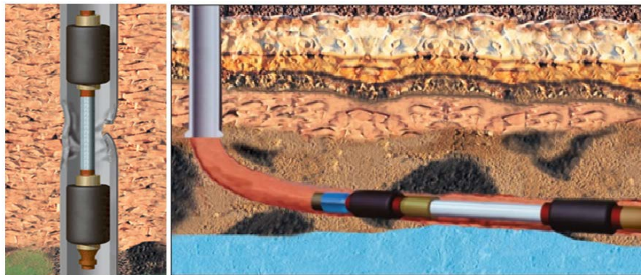
Use of scab liners to reduce excessive sanding.
